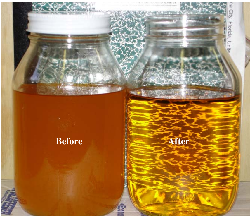
Water Washed Biodiesel before and after a PD206 polishing column.
